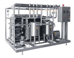
Sterilizing system process many kinds of liquid products, like fruit juice, jam, concentration juice, milk, beverage etc, the temperature can be adjustable according to the production process.
